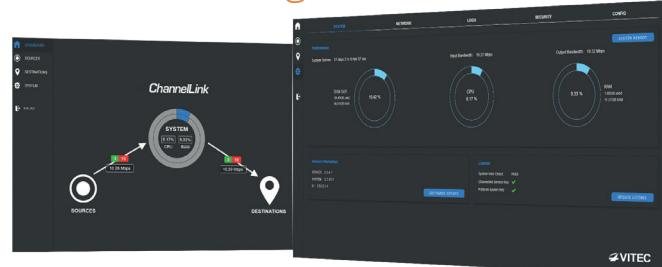
ChannelLink acts as a central IP hub for efficiently and reliably distributing live content from anywhere. ChannelLink can process a large number of input streams protocols (including RTSP for IP camera support) and translate them into a multicast or unicast MPEG Transport Stream over UDP (UDP TS) or an SRT-protected stream, while maintaining the all-important KLV/STANAG 4609 compliant metadata.
